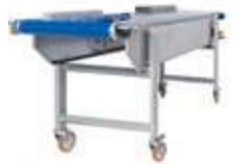
In- & outfeed conveyors
