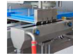
Blade cleaning and washing unit
