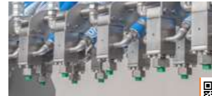
Spray bridge with adjustable spray guns
